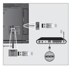
Connect Grundig WiFi USB dongle to the »USB« or »USB HDD« socket of your television in order to connect the television to a wireless network.
